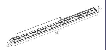
Connection type: Self-clamping block Range of sections of wires used [mm<sup>2</sup>]: 0,5÷2,5 IP class: 20 UGR: <17
