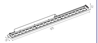
**Enclosure material**: steel, plastic **Connection type**: Self-clamping block
